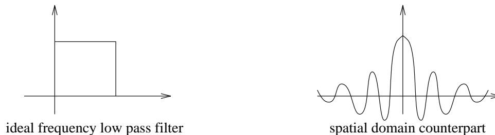
Figure 5: Transfer function for an ideal low pass filter.
